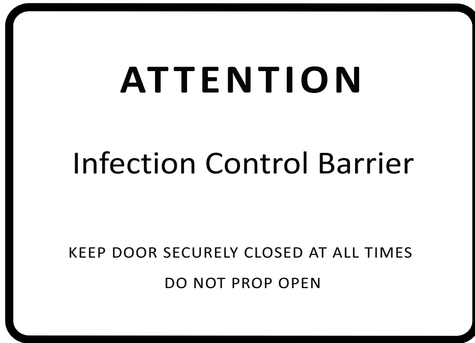
Figure E.6 Preventive measures II to IV infection control dust barrier signage (See Clauses 7.3.2.2 and 7.3.3.)
