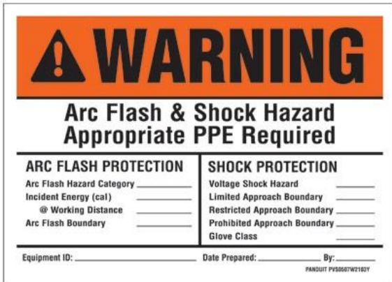
Figure 3 Sample Detailed Warning Label for Arc and Shock Flash
