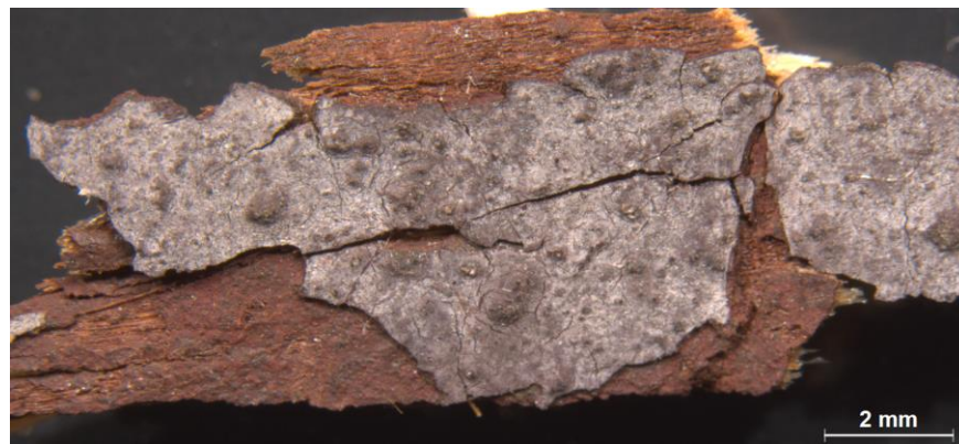
Figure 1: Micrograph of a fragment of paint adhered to the wood substrate. The top layers of paint have flaked off in numerous areas and the top surface is covered with a white bloom.
