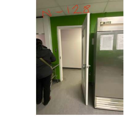
PHOTO 6: REMOVE EXISTING DOOR AND FRAME AND WIDEN OPENING.
