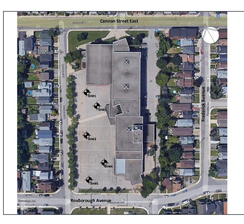
LEGEND **Borehole Location** Υ<sub>BH#</sub> NOTES 1. This drawing should be read in conjunction with SOIL-MAT ENGINEERS & CONSULTANTS LTD. Report No. SM 231080-G 2. Borehole locations are approximate. SOIL-MAT ENGINEERS & CONSULTANTS LTD. **Proposed Pavement** Reconstruction 1292 Cannon Street East Hamilton, Ontario Borehole Location Plan Project No. SM 231080-G Date: February 2024 Drawn: RM
