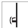
LBE 1 Lever, blank escutcheon KBE Knob, blank escutcheon Always operable (no cylinder)
