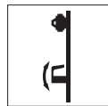
L Lever K Knob Key locks and unlocks Rim and 1 1/4" mortise cylinder Handed, reversible lever Electrified lever operation available
