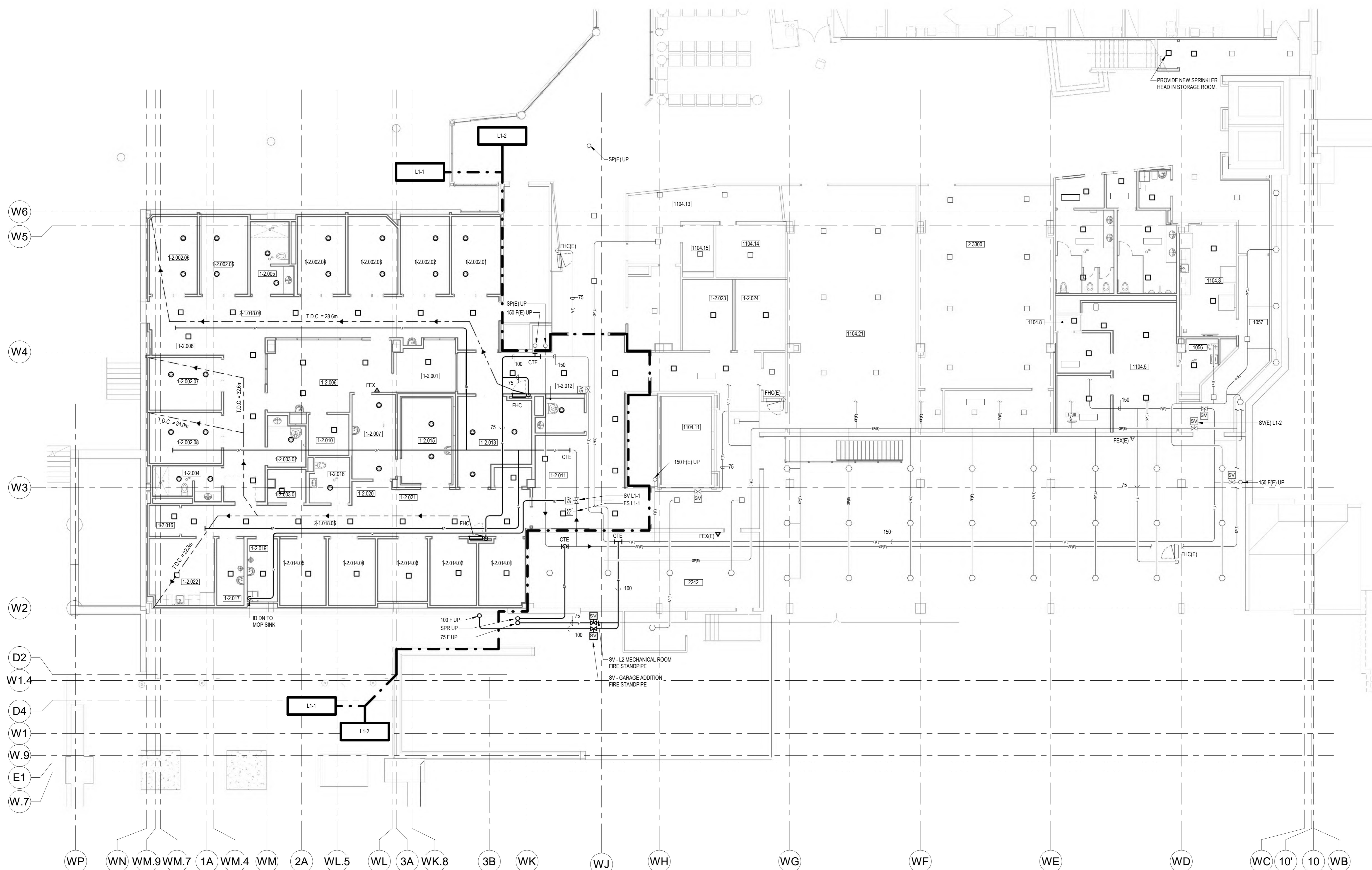
PHASE 1 - PART LEVEL 1 FLOOR PLAN - FIRE PROTECTION SCALE: 1 : 100 NOTES: 1. PROVIDE A WET PIPE SPRINKLER SYSTEM TO NFPA 13 TO COMPLETELY PROTECT ALL AREAS OF THE BUILDING AS SHOWN. 2. SPRINKLER IN STAIRS AND SHAFTS NOT SHOWN. PROVIDE COVERAGE IN ACCORDANCE WITH NFPA 13 AND OBC.
