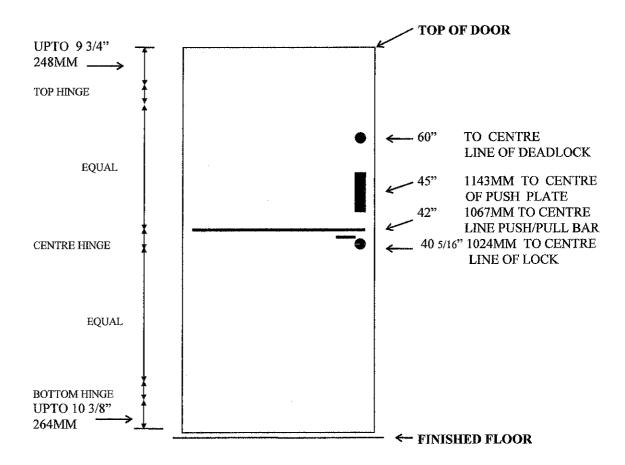
ALL HARDWARE MOUNTING LOCATIONS SHALL BE AS PER LOCATIONS DIAGRAM AND HELD CONSISTENT THROUGHOUT THE PROJECT, UNLESS INDICATED ELSEWHERE IN THE ARCHITECTS DRAWINGS, FINISHING HARDWARE SCHEDULE OR AS DIRECTED BY
