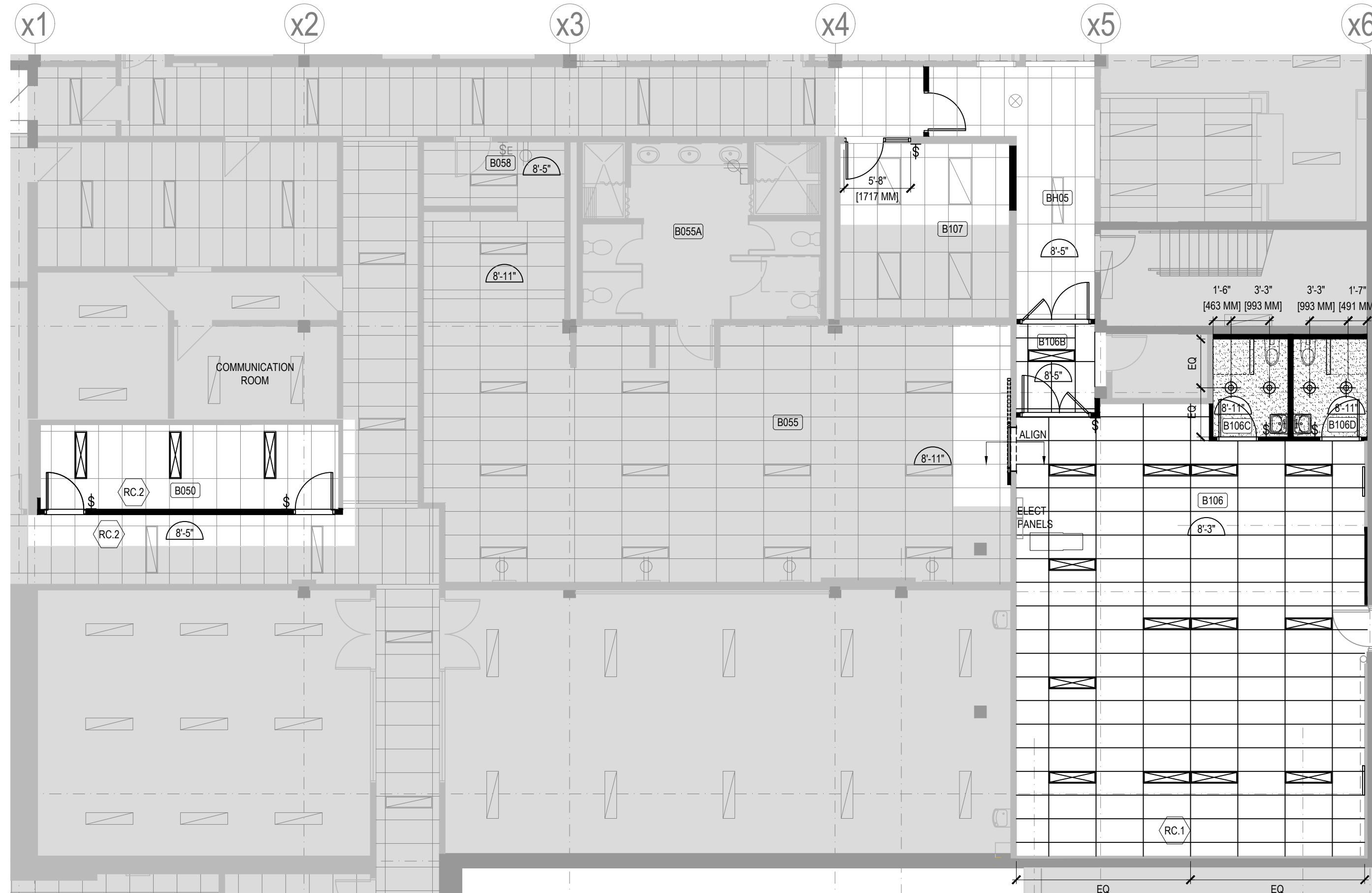
2 REFLECTED CEILING PLAN ID2 SCALE: 1/8" = 1'-0"
