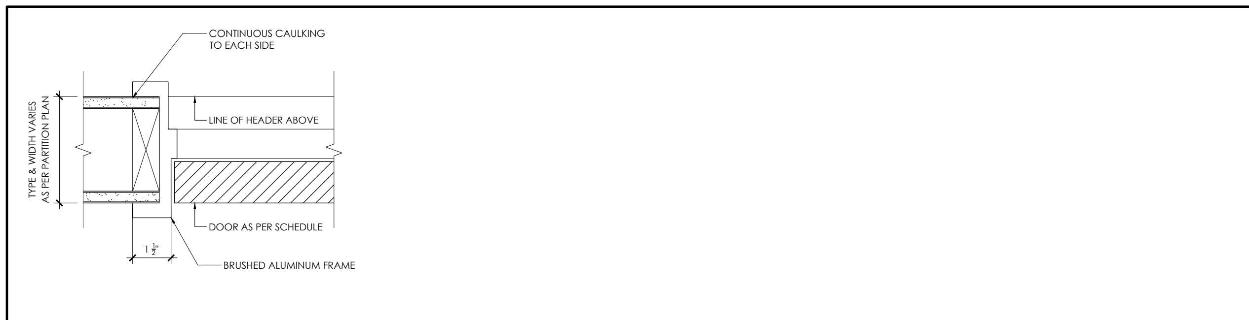
4 TYPICAL HEADER & JAMB DETAILS 3" = 1'-0"
