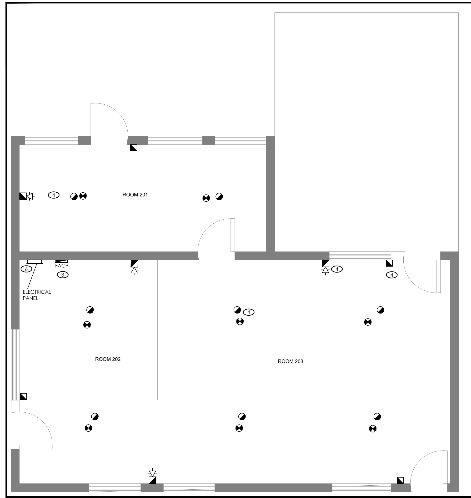
1 STORAGE BUILDING FIRE ALARM PROPOSED PLAN SCALE: 1:100
