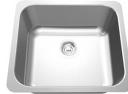
Without faucet ledge, 18 gauge Type 304 Stainless steel Polished to #4 satin finish, Center back waste location, 38 mm (1-1/2") (DN38) brass tailpiece, 89 mm (3-1/2") crumb cup strainer, waste fitting included, Undercoated to reduce condensation and resonance,
