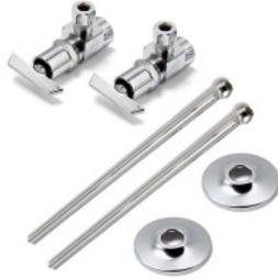
☒ **LFCK165LK** Lead Free, with Chrome-plated finish, Pipe to compression connection, 3/8" I.P.S x 3/8" O.D connection, Shallow wall flange, Loose key handle, Full turn brass stem, 305 mm (12") chrome-plated risers, Purple EPDM peroxide cured washers,
