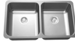
Without faucet ledge, 18 gauge Type 304 Stainless steel Polished to #4 satin finish, Center back waste location, 38 mm (1-1/2") (DN38) brass tailpiece, 89 mm (3-1/2") crumb cup strainer, waste fitting included, Undercoated to reduce condensation and resonance,
