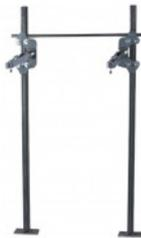
☒ **WCA-411** WCA-411/WCA-411-WC, Single floor-mounted lavatory carrier with concealed arms, For concealed arm carrier, adjustable arms, epoxy coated cast iron, integral welded feet, upper tie rod, Heavy gauge steel offset uprights, basin locking device, Plated hardware, levelling screws.
