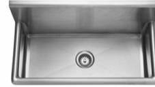
203 mm (8") centerset, 14 gauge Type 304 Stainless steel Polished to #4 satin finish, With 152 mm (6") high backsplash, Radius coved bowl corners and rolled radius rim, Center waste location, 38 mm (1-1/2") (DN38) brass tailpiece, 89 mm (3-1/2") crumb cup strainer,
