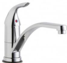
☒ **430-ABCP** Counter mounted, Manual, Single handle, Sink faucet, Polished chrome finish, Single hole centerset, Lead Free ANSI/NSF 61 compliant, ECAST® brass construction, Ceramic cartridge with volume control, 5.7 LPM (1.5 GPM) maximum flowrate, Pressure compensating Econo-Flo™ non-aerated laminar spray outlet, Tubular cast brass spout, 229 mm (9") spout reach, 146 mm (5-3/4") high, 108 mm (4-1/4") lever handle, 13 mm (1/2") NPSM supply inlet, Includes hot limit safety stop.
