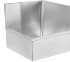
Without faucet ledge, 16 gauge Type 316 Stainless steel Polished to #4 satin finish, With 305 mm (12") high backsplash and integral corner splashguard, Radius coved bowl corners, Includes one piece wall hangers, Center waste location, 51 mm (2") I.P.S. grid drain, Undercoated to reduce condensation and resonance,
