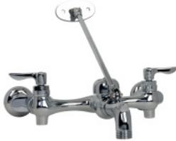
☒ **8354112.002** Wall-hung, Manual, Two handles, Mop sink faucet, Polished chrome finish, 152 - 254 mm (6" - 10") adjustable centerset, Brass construction, Integral check valve, Ceramic disc cartridge, no flow restrictor, 37.8 LPM (10 GPM) @20 PSI, Threaded hose end, Cast brass spout with bucket hook, 248 mm (9-3/4") spout reach, Top brace, Vandal-resistant lever handles, 13 mm (1/2") female inlet.
