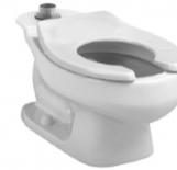
Toilet, Floor mounted with floor outlet, Toilet operates in the range of 4.8 to 6.0 LPF (1.28 - 1.6 GPF), White finish Vitreous china, Junior bowl, 260 mm (10-1/4") rim height for toddlers, Minimum 254 mm (10") rough-in from wall to the center of waste outlet, Siphon jet flush action, 38 mm (1-1/2") top spud, Flush valve by others, Fully-glazed trapway, Toilet seat not included, Two (2) colour-matched bolt caps with retainers (481310-100), Consisting of:
