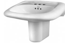
Wall-hung Lavatory, Vitreous china, EverClean® antimicrobial surface, White finish, 102 mm (4") centerset. Rear overflow, Faucet ledge with recessed self-draining deck, For concealed arm or wall support, Acrylic shroud, conceals control box and thermostatic mixing valve (0097000), Soap dispenser, When installed with a below deck electronics faucet which has the control box, the accessories will not fit under the shroud and will need to be installed outside the shroud,
