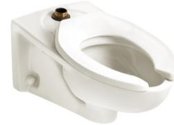
Toilet, Wall-hung with wall outlet, Toilet operates in the range of 4.2 to 6.0 LPF (1.1 - 1.6 GPF), White finish Vitreous china, EverClean® antimicrobial surface, Elongated bowl, Concealed trapway design, Direct-fed siphon jet flush action, 38 mm (1-1/2") top spud, Flush valve by others, Fully-glazed 54 mm (2-1/8") trapway, Static load rating of 454 kg (1000 lb), this product is not recommended for bariatric use, Condensation channel, Toilet seat not included, Consisting of:
