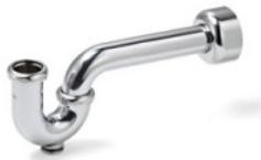
☒ **8902CB** Cast brass body material, Chrome-plated finish, Professional line box flange, 292 mm (11-1/2") length, With cleanout plug, Steel box flange, Neoprene gasket, Slipnuts, 17 gauge seamless tubular wall bend
