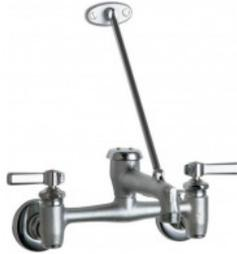
☒ **897-RCF** Wall-hung, Manual, Two handles, Mop sink faucet, Rough chrome plated finish, 194 - 213 mm (7-5/8" to 8-3/8") adjustable centerset, Round wall escutcheons, Brass construction, Adjustable supply arms, 1/4 turn ceramic cartridge, No flow restrictor, Threaded hose end, Spout with pail hook, 146 mm (5-3/4") spout reach, 273 mm (10-3/4") high, Top brace, 60 mm (2-3/8") lever handle with indexed buttons, Atmospheric vacuum breaker is not intended for continuous pressure applications.
