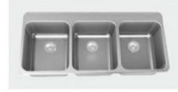
Single hole centerset, With faucet ledge, 18 gauge Type 304 Stainless steel Polished to #4 satin finish, Factory installed EZ TORQUE™ fasteners, Factory applied rim seal, Center back waste location, 38 mm (1-1/2") (DN38) brass tailpiece, 89 mm (3-1/2") crumb cup strainer, waste fitting included, Undercoated to reduce condensation and resonance,
