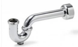
☒ **8912CB** Heavy cast brass, Adjustable p-trap, 292 mm (11-1/2") length, With cleanout plug, Steel box flange, Neoprene gasket, Seamless tubular brass bend, Slipnuts
