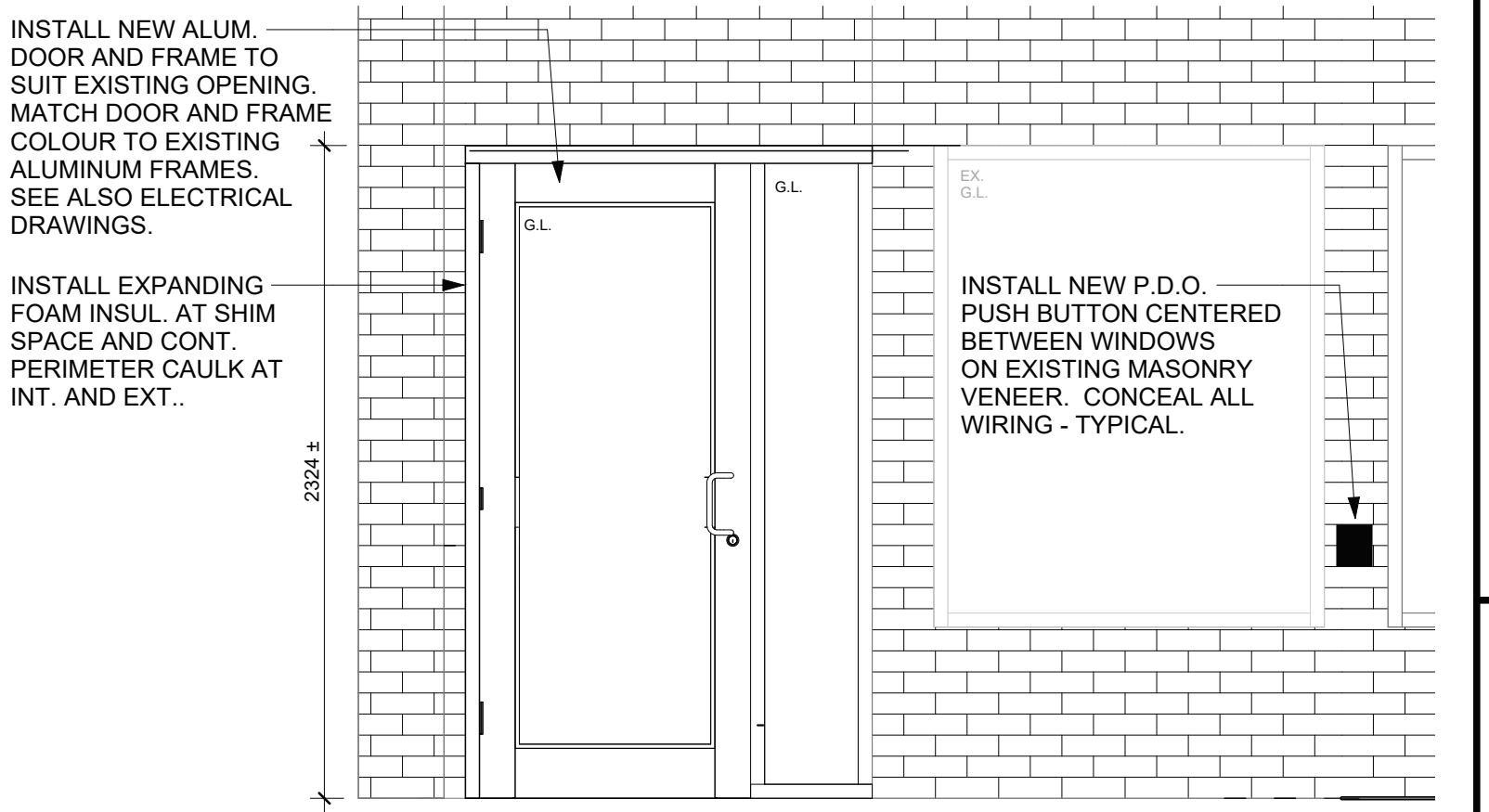
9 PARTIAL FRONT ENTRANCE ELEVATION 1 : 25
