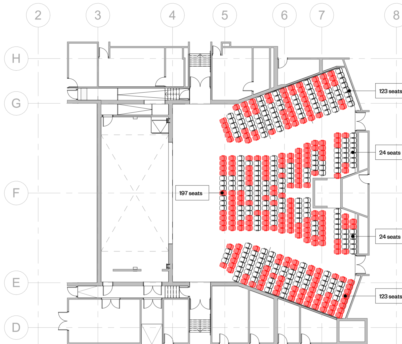
1 Level 01 - Existing Auditorium Seating Condition 1/16" = 1'-0"
