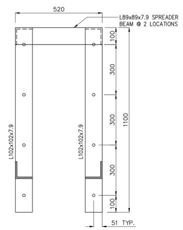
5 CABLE TRAY SUPPORT BRACKET TYP. SECTION
