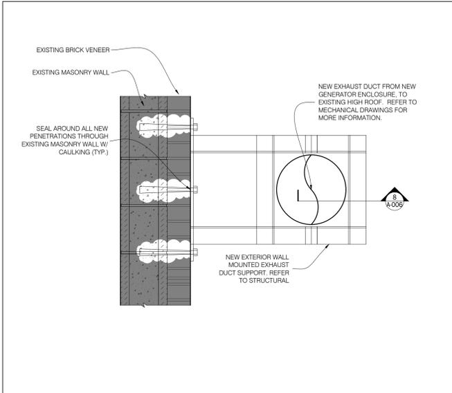
7 EXHAUST PIPE SUPPORT PLAN DETAIL
