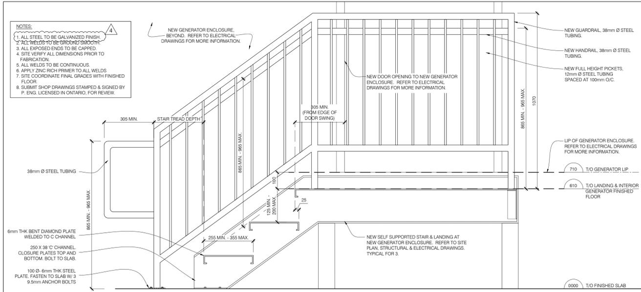
2 STAIR DETAIL AT GENERATOR ENCLOSURE - TYPICAL
