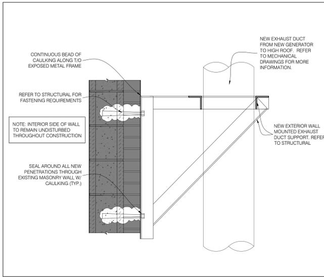
8 EXHAUST PIPE SUPPORT SECTION DETAIL
