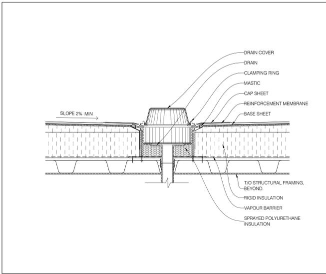
10 ROOF DRAIN DETAIL
