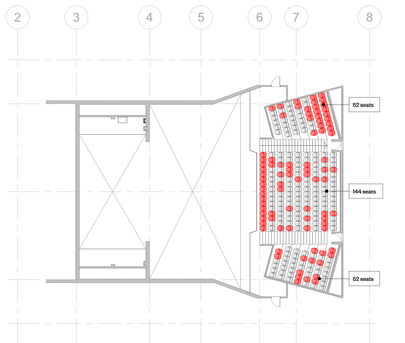
2 Level 02 & 03 - Existing Balcony Seating Condition 1/16" = 1'-0"
