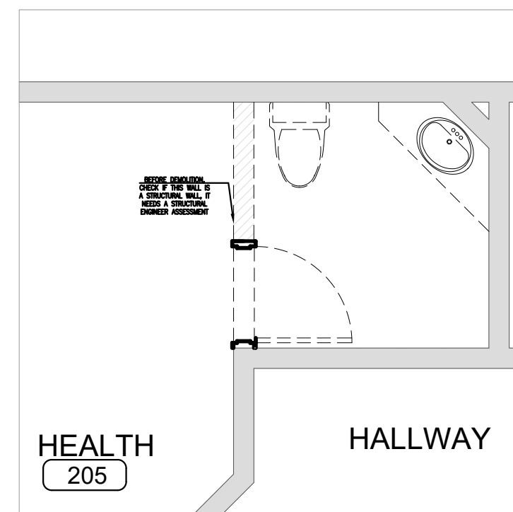
EXISTING AND DEMOLITION WASHROOM LAYOUT SCALE 1/50
