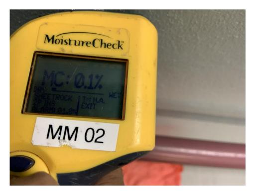
Photo 1: Moisture reading indicated the wall was dry at the time of assessment
