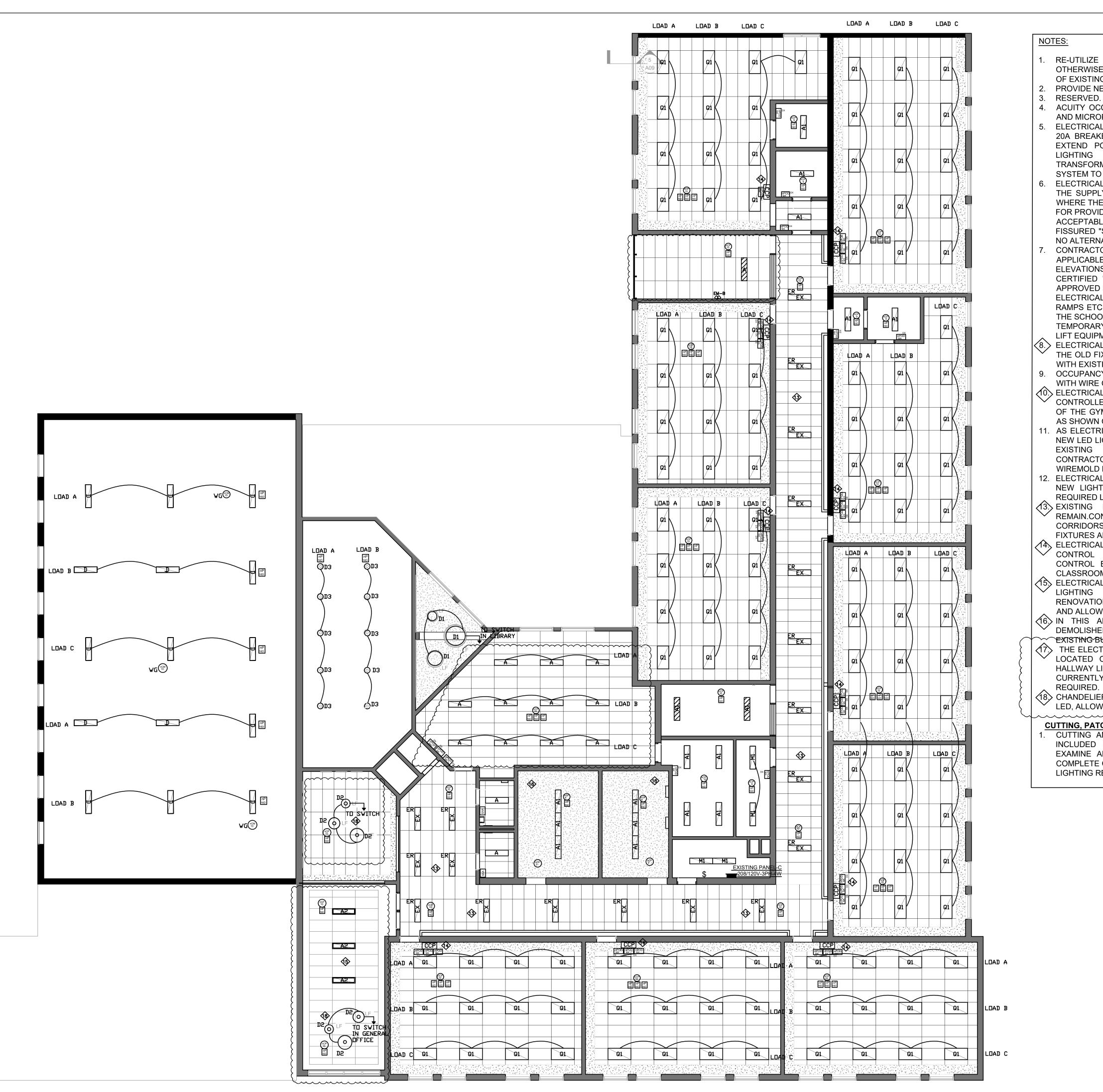
RE-UTILIZE EXISTING LIGHTING CIRCUITS UNLESS NOTED OTHERWISE. ELECTRICAL CONTRACTOR TO VERIFY CAPACITY OF EXISTING LIGHTING CIRCUIT PRIOR TO INSTALLATION.
