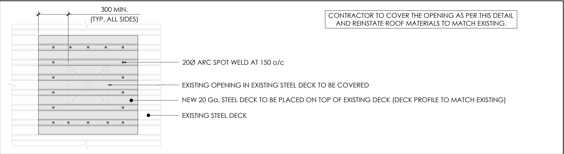
01 S.01 TYPICAL ROOF OPENING REPAIR DETAIL Scale 1:20
