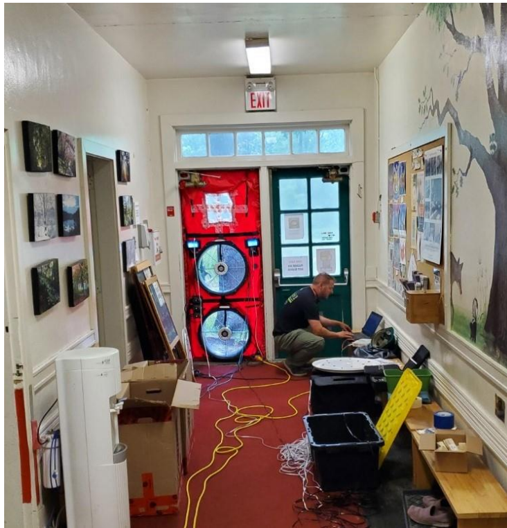
Figure 5: Blower door fan set up at the ground floor entrance on the north-west side.
