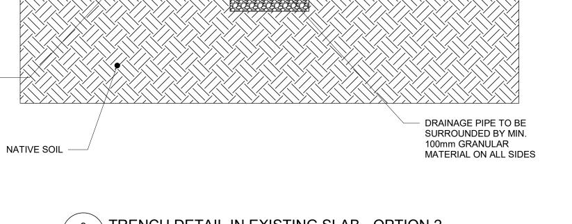
3 TRENCH DETAIL IN EXISTING SLAB - OPTION 2 S5101 | Scale: 1:10
