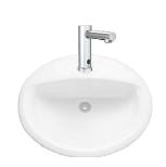
COUNTER-MOUNTED SINK: (BARRIER FREE USE) L2H WHITE, FOR BARRIER FREE USE, SELF-RIMMING WITH SEALANT, OVERFLOW, DRILLED FOR 100 MM SUPPLY FITTING. AMERICAN STANDARD "AQUALYN" #0475.047.020 518 X 441 MM
