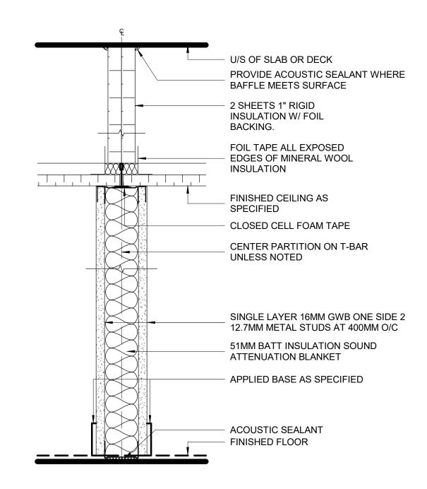
NOTE: ANCHOR TOP TRACK TO T-BAR WITH CLIPS OR FASTENERS DO NOT SCREW TO MAIN T's
