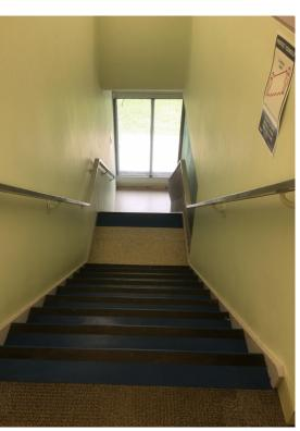
PHOTO 1: REMOVE EXISTING TEXTURE WARNING STRIP ON EACH STEP
