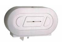
TOILET TISSUE DISPENSER: TPD SURFACE-MOUNTED TWIN JUMBO-ROLL B-2892: 18-8, TYPE-304, 20-GAUGE (1.0MM) STAINLESS STEEL WITH SATIN-FINISH. EQUIPPED WITH A TUMBLER LOCK KEYED LIKE OTHER BOBRICK WASHROOM ACCESSORIES.
