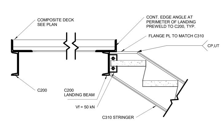
TYPICAL SECTION AT UPPER LANDING D2200 / Scale: 1:10
