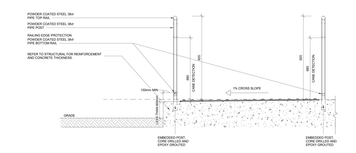
3 SECTION OF GUARDRAIL FOR RAMP AT GRADE DIFFERENCE LESS THAN 600 MM D1403 Scale: 1:10
