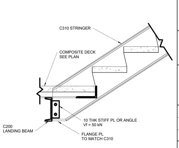
11 TYPICAL SECTION AT LOWER LANDING ∖ D2200 / Scale: 1 : 10
