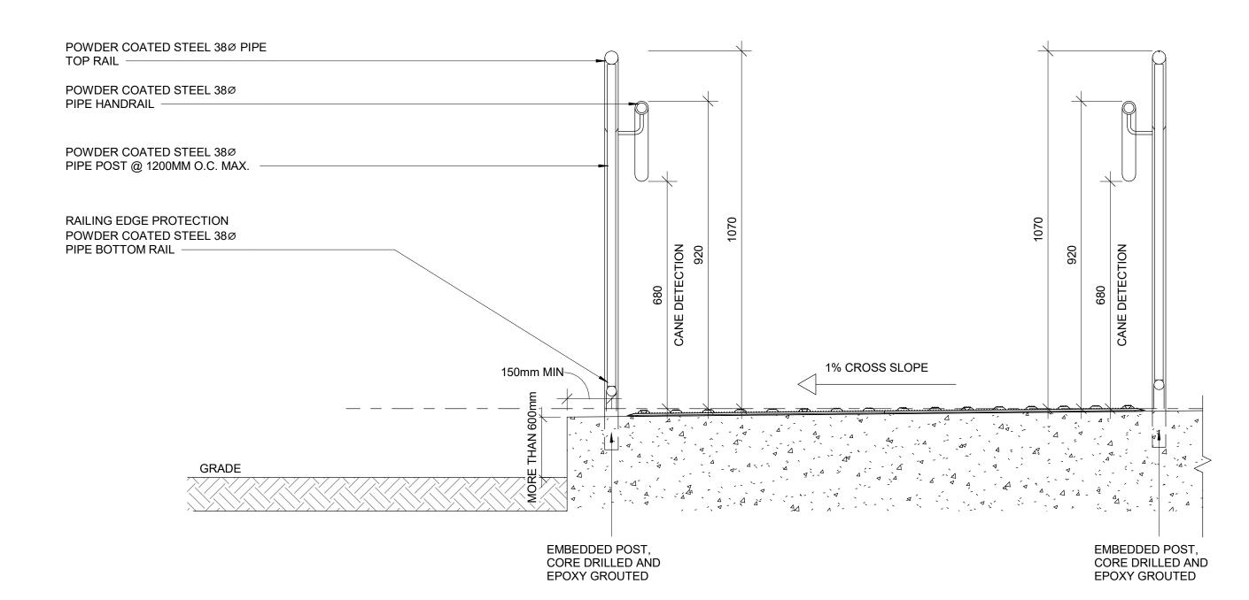
1 ELEVATION OF GUARDRAIL FOR RAMP AT GRADE DIFFERENCE MORE THAN 600 MM D1404 Scale: 1:10
