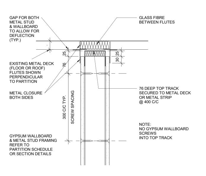
4 HEAD FULL HEIGHT DRYWALL PARTITION - NON RATED D1501 Scale: 1:5
