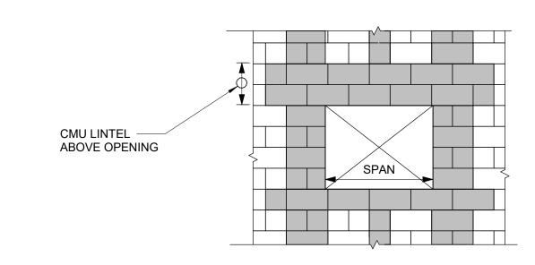
4 OPENING IN NEW MASONRY WALL D2300 / Scale: 1:20
