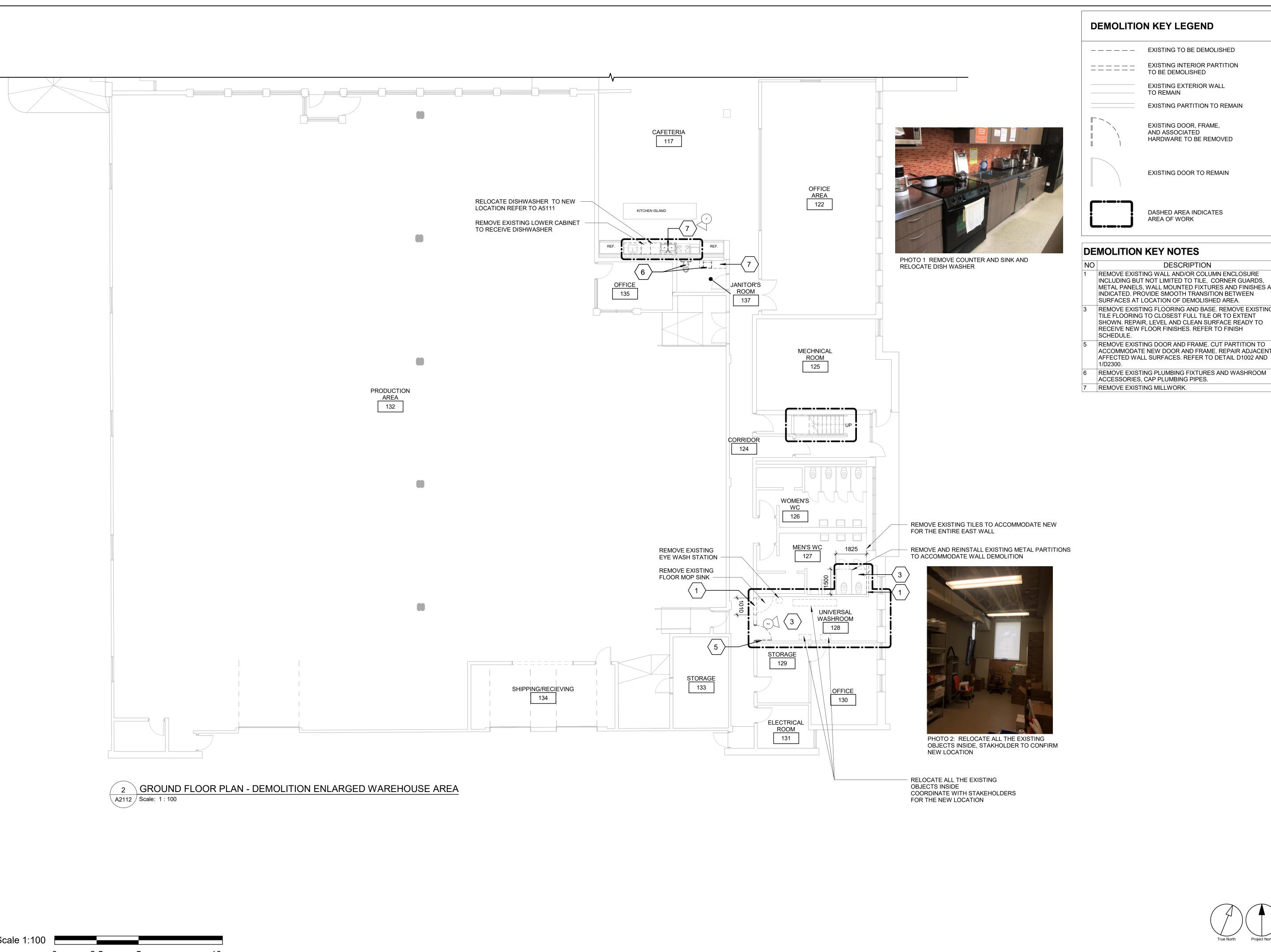
REMOVE EXISTING WALL AND/OR COLUMN ENCLOSURE INCLUDING BUT NOT LIMITED TO TILE, CORNER GUARDS, METAL PANELS, WALL MOUNTED FIXTURES AND FINISHES AS INDICATED. PROVIDE SMOOTH TRANSITION BETWEEN
