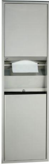
PAPER TOWEL DISPENSER AND WASTE RECEPTACLE: PTD/WR (R) RECESSED CONVERTIBLE B-3940: 18-8, TYPE 304, HEAVY-GAUGE STAINLESS STEEL. EXPOSED SURFACES HAVE STAIN-FINISH.
