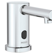
SOAP DISPENSER: SD-2 COUNTER MOUNTED, TOUCH FREE, ONE PIECE, CAST BRASS CONSTRUCTION ABOVE DECK, SINGLE MOUNT FOAM SOAP DISPENSER WITH ADJUSTABLE SENSOR. MOEN, MODEL NO. 8560
