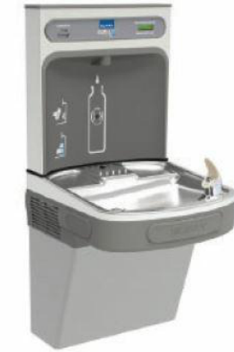
DRINKING FOUNTAIN: DF EZSDWSLK GALVANIZED STEEL WALL MOUNTED, WHEELCHAIR TYPE WATER COOLER WITH STAINLESS STEEL TOP, FRONT AND SIDE MOUNTED PUSH TO OPERATE LEVER(S), SENSOR, TOUCHLESS ACTIVATION WITH AUTO SHUT OFF BOTTLE FILLER, FLEXI-GUARD SAFETY BUBBLER, AND TRAP PACKAGE.
