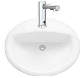
COUNTER-MOUNTED SINK: (BARRIER FREE USE) L2H WHITE, FOR BARRIER FREE USE, SELF-RIMMING WITH SEALANT, OVERFLOW, DRILLED FOR 100 MM SUPPLY FITTING. AMERICAN STANDARD "AQUALYN" #0475.047.020 518 X 441 MM
