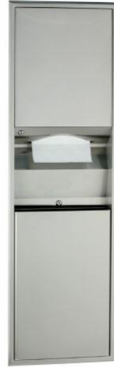
PAPER TOWEL DISPENSER AND WASTE RECEPTACLE: PTD/WR (R) RECESSED CONVERTIBLE B-3940 : 18-8, TYPE 304, HEAVY-GAUGE STAINLESS STEEL. EXPOSED SURFACES HAVE STAIN-FINISH.
