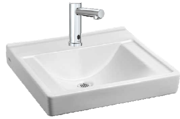
WALL MOUNTED SINK: (BARRIER FREE USE) L1H DECORUM WALL HUNG LAVATORY WITH EVERCLEAN 9024.001EC.020 - VITREOUS CHINA, WHITE FINISH, WITH SINGLE FAUCET HOLE AND OVERFLOW
