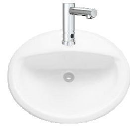
COUNTER-MOUNTED SINK: L1 WHITE, SELF-RIMMING, REAR/FRONT OVERFLOW, DRILLED FOR 100 MM SUPPLY FITTING. AMERICAN STANDARD "AQUALYN" #0475.047.020 518 X 441 MM
