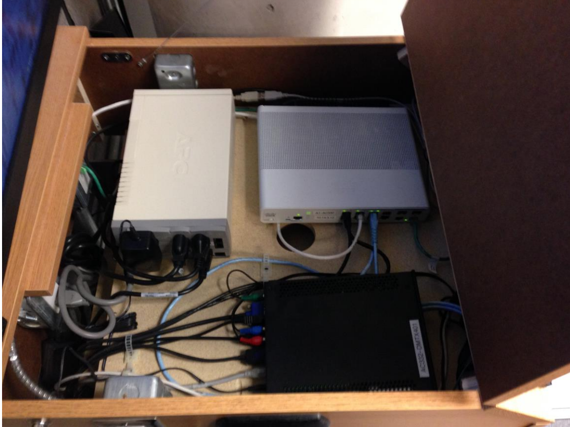
Fig 3.0.3: Top view of a clean TSJr installation – note presence of UPS and Network Switch.
