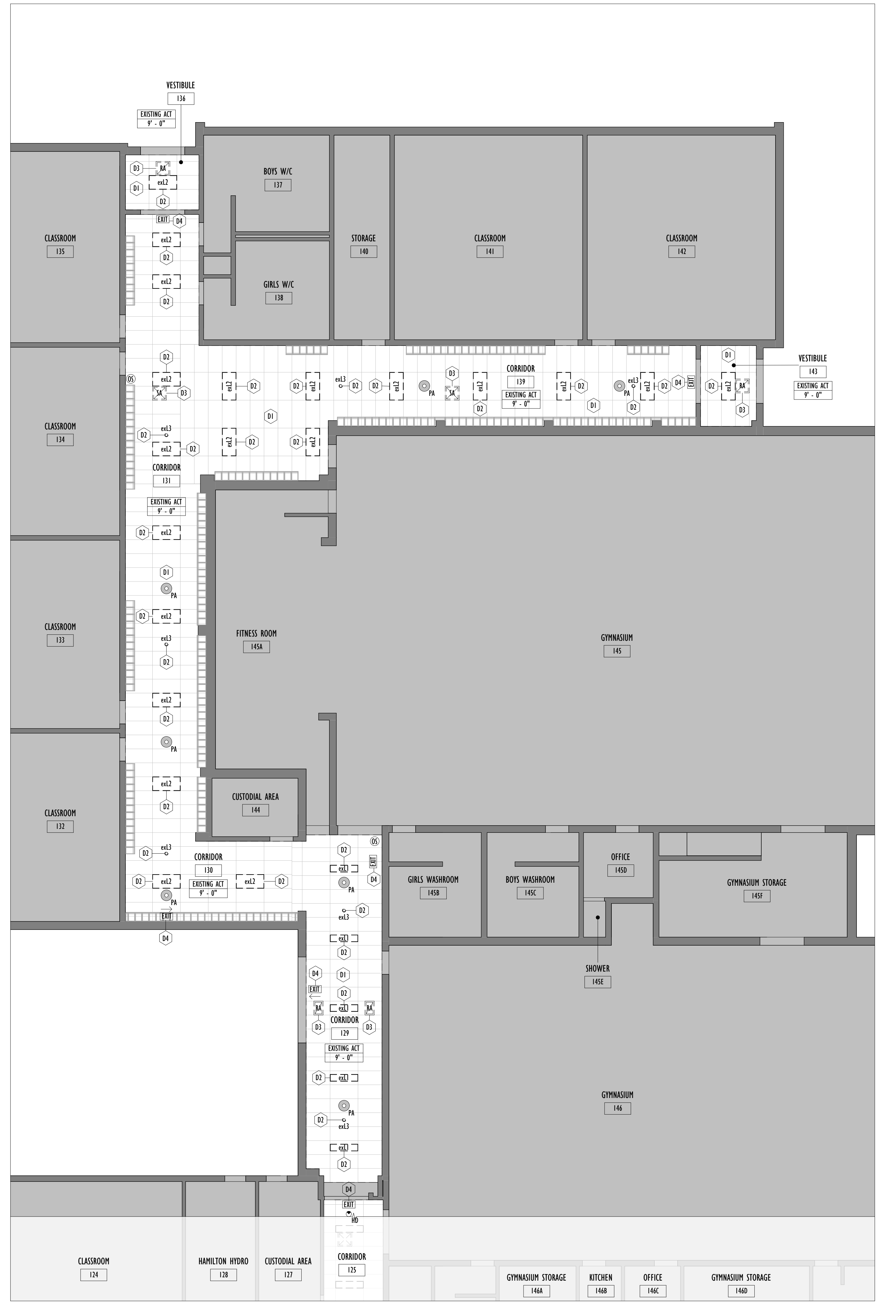
2 DEMOLITION PARTIAL GROUND FLOOR RCP - C Scale: 1 : 100
