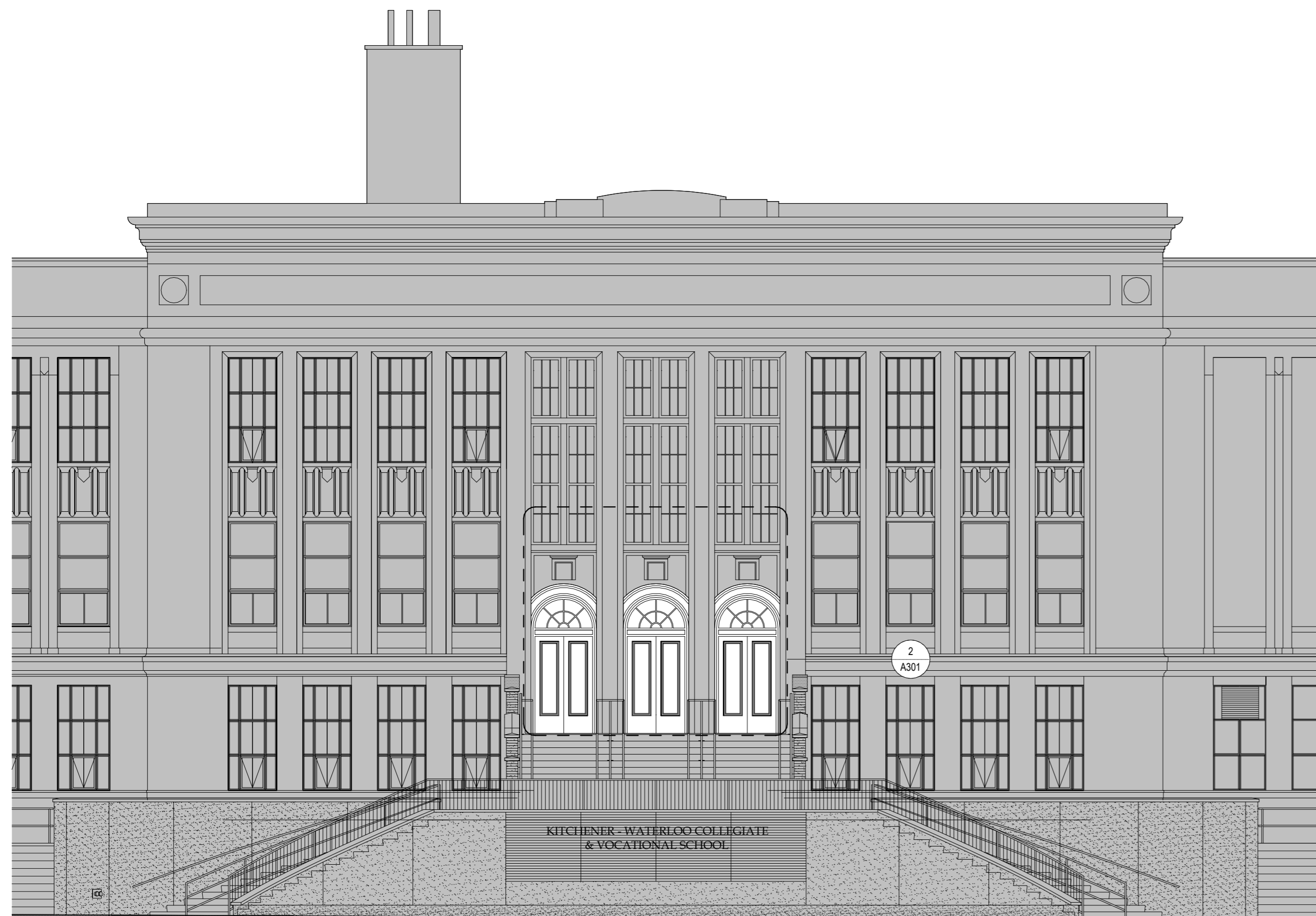
1 DOOR RESTORATION - PARTIAL ELEVATION A301 Scale: 1 : 100
