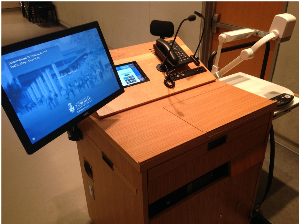
Fig 2.1.1: Full Teaching Station angled top view. Note the PC installed on its side on front shelf area giving user access to the USB slots and DVD drive.
